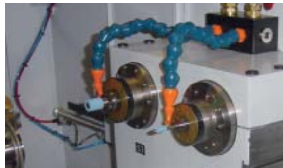
The CT-450 comes fitted with two FISCHER MFM 1242/60 and MFM 1290/90 internal grinding spindles as standard.
